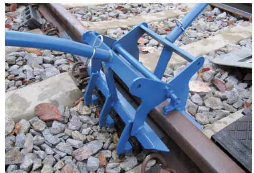
**Final check: The damper is in final position if the fixing pins are protruding at an approximately equal length.**
